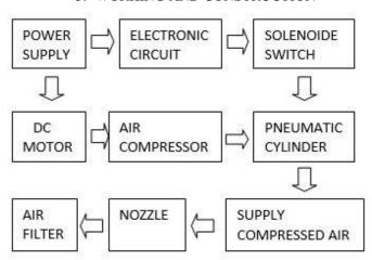
From this block diagram we get information about the component and how they are link up with each other. We take power supply from electric board for DC motor, Air compressor and electronic circuit by single wire. In electronic circuit there are three components.
